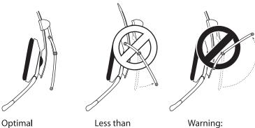
ideal **Excessive twisting** may damage internal wiring!
