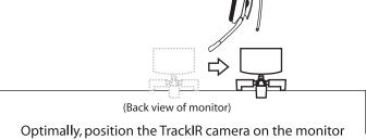
so that it is centered with the TrackClip PRO's LEDs.
